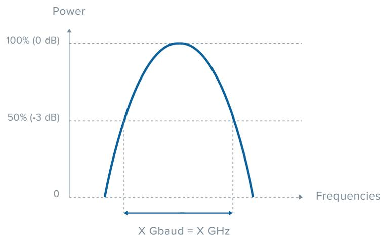
**FIGURE 3** — Symbol Rate and Channel Width
