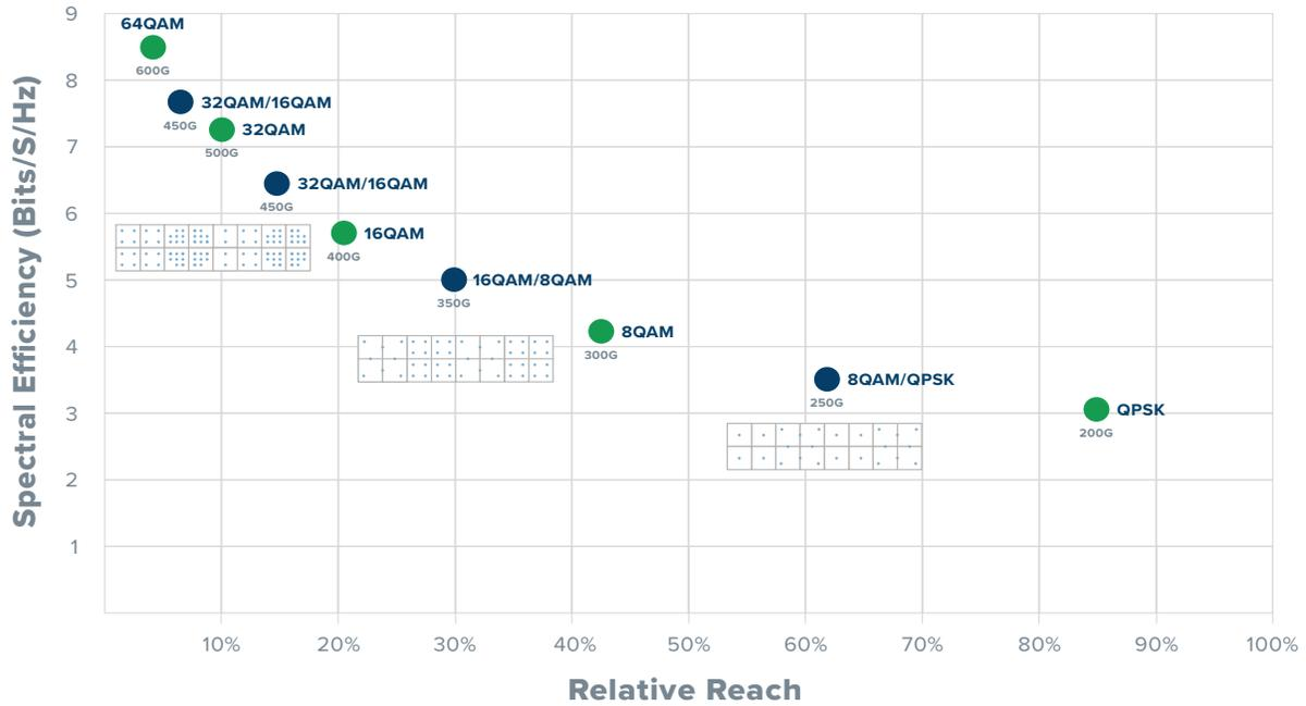
**FIGURE 11** – 69 Gbaud with Hybrid Modulation
