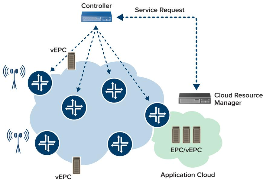
FIGURE 8 – SDN Control in an Access and Aggregation Network for Real Time Access to Virtualized Resources
