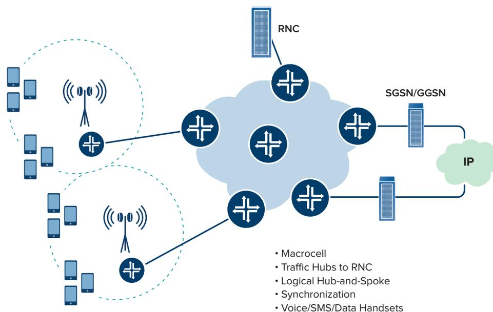
FIGURE 2 – Traditional Hub-and-Spoke Mobile Network Architecture
