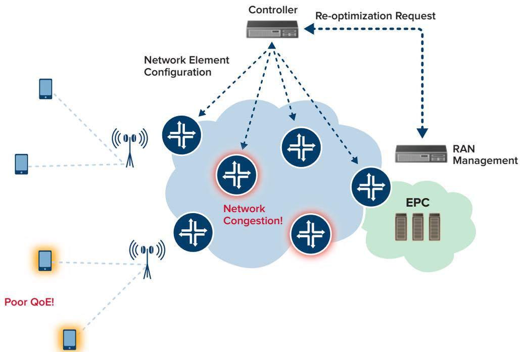
FIGURE 6 – Improved MBH Network Utilization under SDN Control
