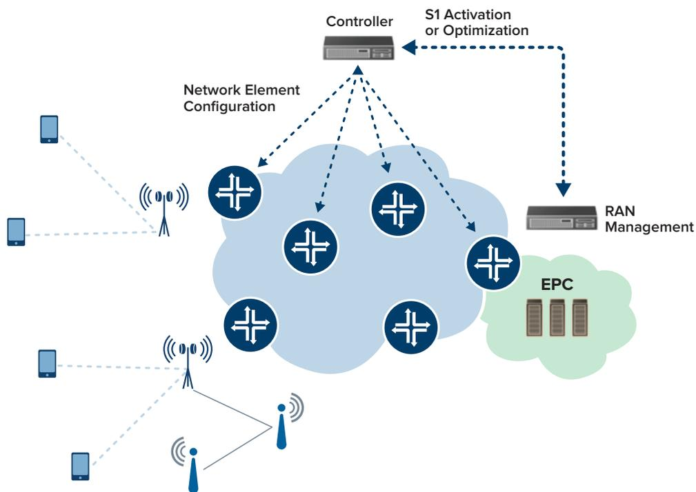
FIGURE 5 – SDN Automation of S1 Interface Activation and Optimization
