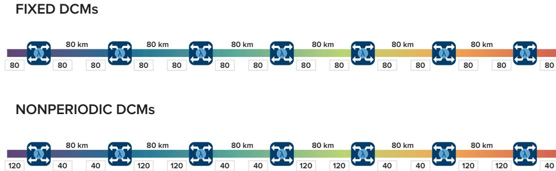
FIGURE 8 – Fixed vs. Nonperiodic Chromatic Dispersion Compensation
