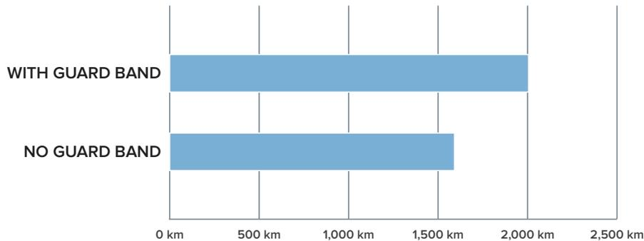
FIGURE 7 – The impact of guard bands on Coriant CloudWave™ Optics 100G reach in 10G/100G long haul networks
