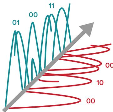
FIGURE 2 – 10G Modulation: Polarization Multiplexed-Quadrature Phase Shift Keying (PM-QPSK)
