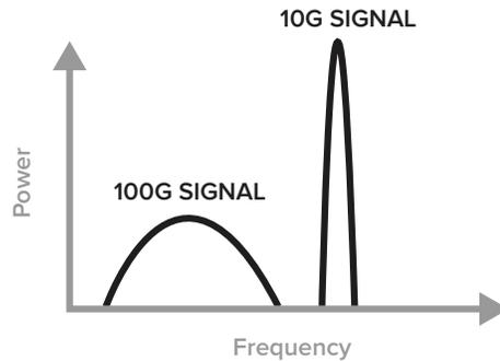
FIGURE 3 – Signal Power Density: 10G vs. 100G
