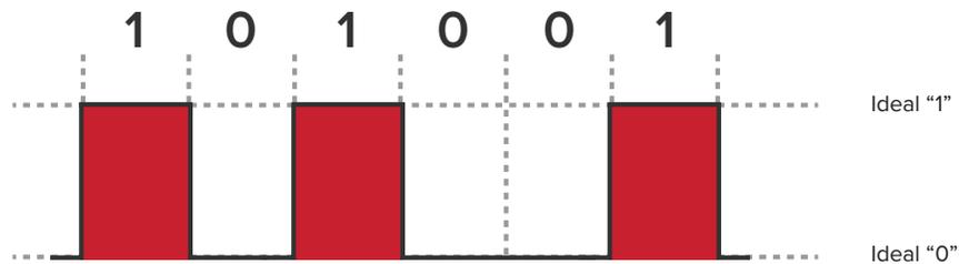
FIGURE 1 – 10G Modulation: On-Off Keying (OOK)
