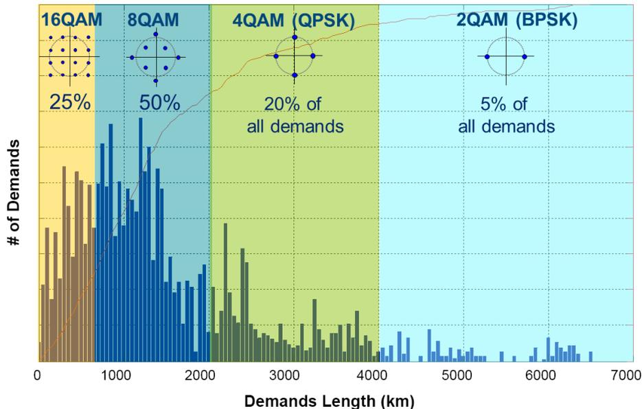
Figure 1: Example of a flexi-rate interface with multiple modulation schemes on a cumulative distribution of demands in core networks with Raman amplification\*
