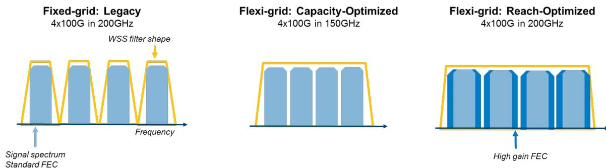
Figure 2: Example of flexi-grid and super-channel use cases
